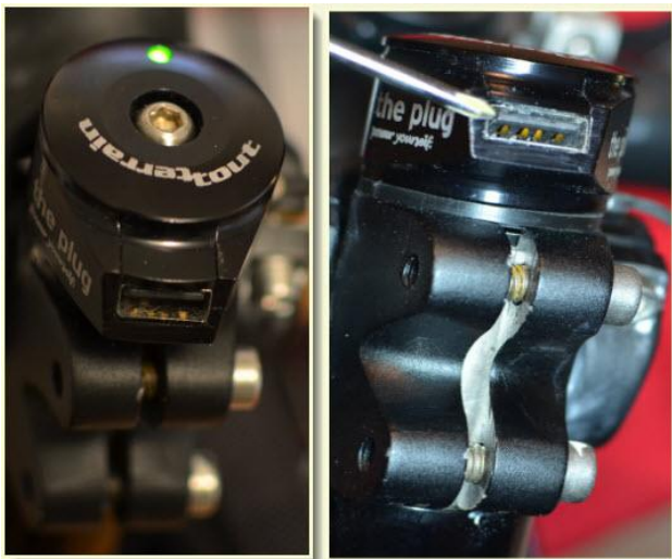
The LED green light is easily seen in daylight. The USB port has a female upper connector as shown in the picture on the right.
