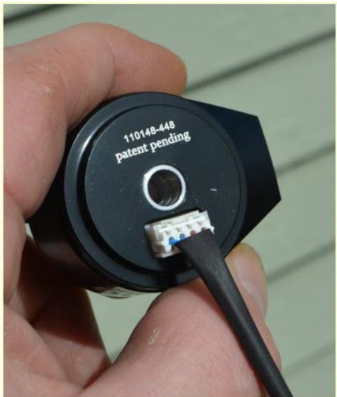
The white molded connector mates and locks into the TopCap's bottom module.
